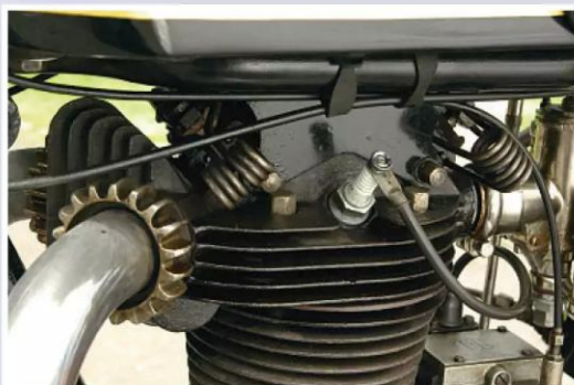
Two sides of a singular engine. OHV, with exposed valve springs and pushrods, as well as some remarkable plumbing
