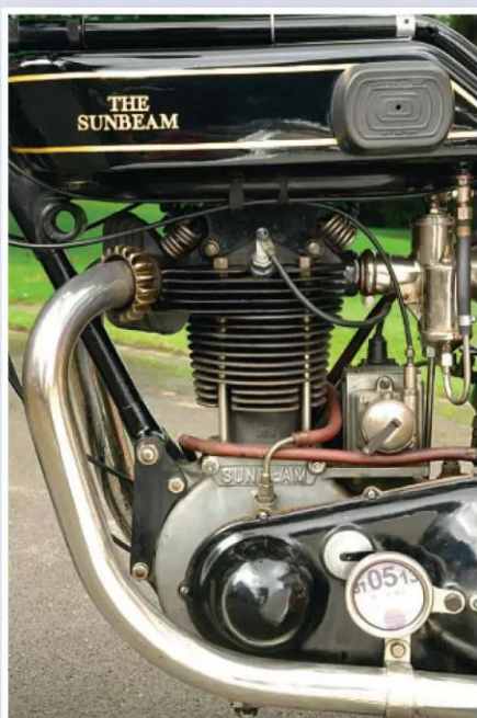
Two sides of a singular engine. OHV, with exposed valve springs and pushrods, as well as some remarkable plumbing
