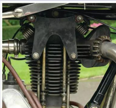
Two sides of a singular engine. OHV, with exposed valve springs and pushrods, as well as some remarkable plumbing
