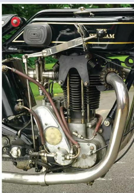
Two sides of a singular engine. OHV, with exposed valve springs and pushrods, as well as some remarkable plumbing
