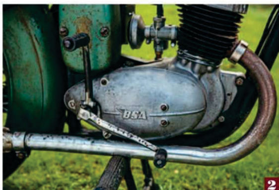
2: From mid-1950 the exhaust pipe was routed above the footrest. Using the kickstart, mounted concentrically with the gearchange, was a pain for big feet.
