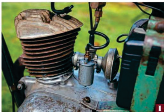
1: Amal 261 carburettor with 'strangler' choke/air filter. The set-up returned over 110mpg.
